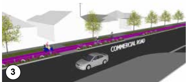
Extended kerb to create 3m bi-directional facility on Commercial Road with minimum 0.6m planted buffer.
