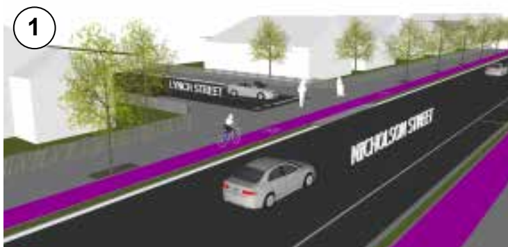
Extended kerbs on both sides of Nicholson Street. Minimum 1.5m raised bicycle lane with minimum 0.6m buffer.
